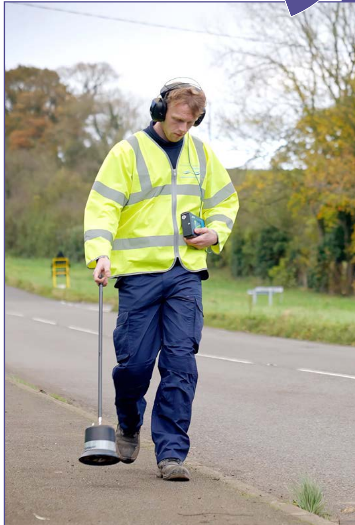
Detecting leaks using a ground microphone.
