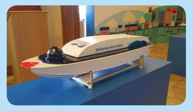
Our unmanned waterborne vehicle is used to conduct bathometric surveys of impounding reservoirs. Using GPS guidance it navigates a predefined grid pattern across the reservoir surface taking a depth reading every second and logging the data along with latitude and longitude coordinates. The data from the survey can be processed to create a 3D model of the reservoir bottom and from this
