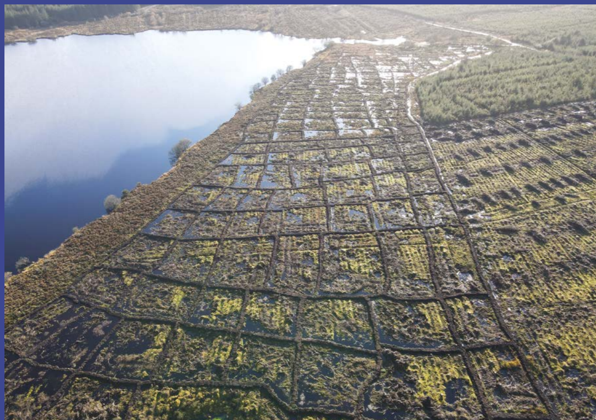
This 10-hectare peatland plot along the shores of Lough Bradan Reservoir, County Tyrone, has been restored using the innovative 'cell bunding' technique.
