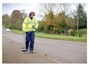
Detecting leaks using a ground microphone.
