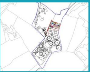
The diagram above shows the layout of the Dungannon wastewater treatment works, County Tyrone (NI Water land ownership outlined in blue) with the new Nereda\* process being installed to the north of the site (marked in colour).
