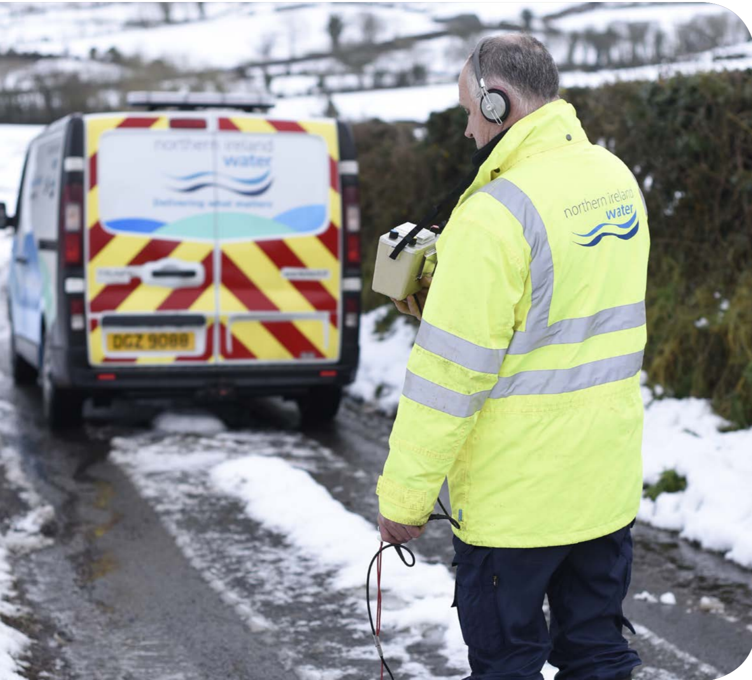
Leakage detection technology being used by a NI Water staff member.
