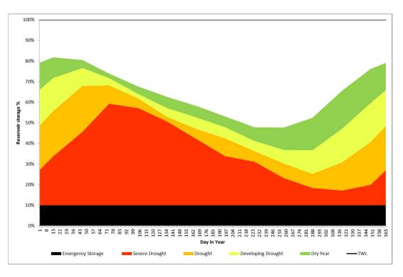
Figure 5.1: Drought Curves Developed for a Reservoir Group
