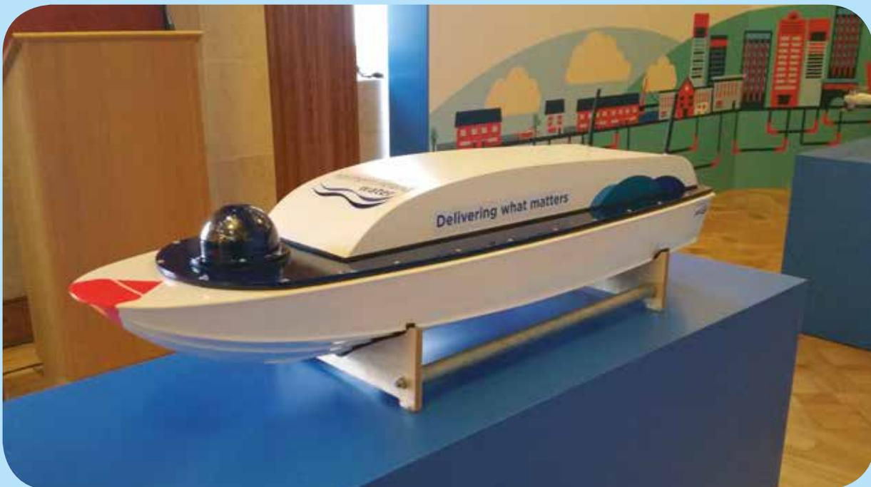
Our unmanned waterborne vehicle is used to conduct bathymetric surveys of impounding reservoirs. Using GPS guidance it navigates a predefined grid pattern across the reservoir surface taking a depth reading every second and logging the data along with latitude and longitude coordinates. The data from the survey can be processed to create a 3D model of the reservoir bottom and from this
