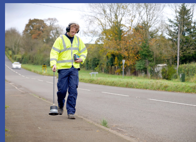
Detecting leaks using a ground microphone.
