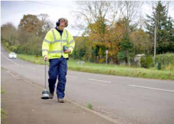
Detecting leaks using a ground microphone.
