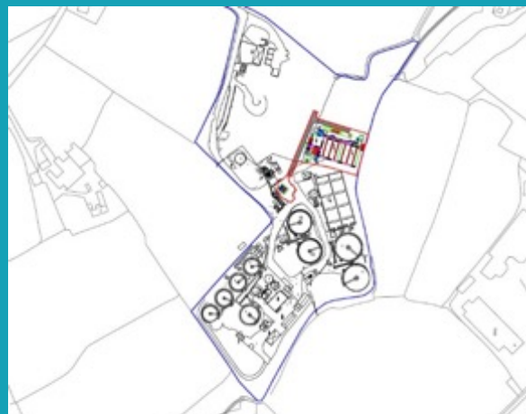
The diagram above shows the layout of the Dungannon wastewater treatment works, County Tyrone (NI Water land ownership outlined in blue) with the new Nereda® process being installed to the north of the site (marked in colour).
