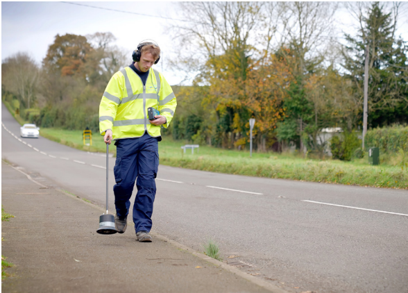
Detecting leaks using a ground microphone.
